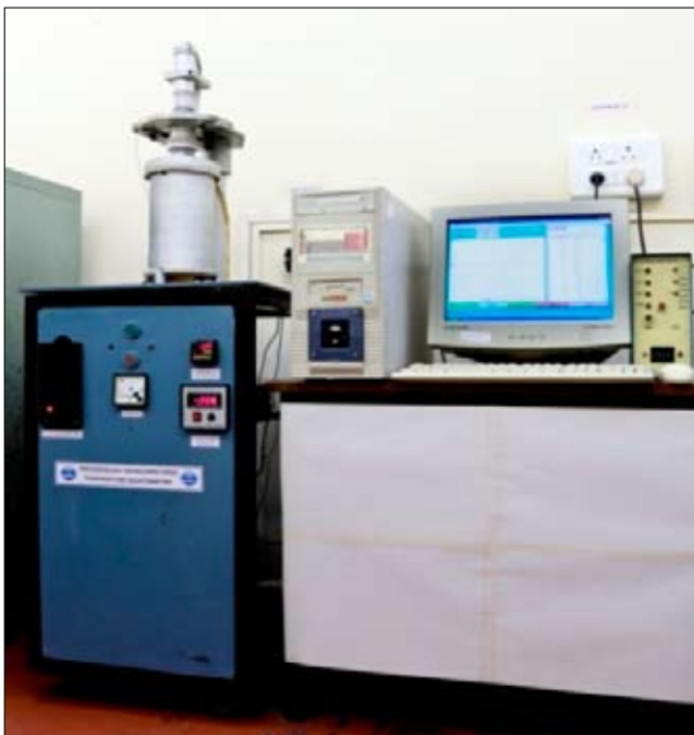
Fig. 24: High Temperature Dilato-meter (RT - 1373 K)
