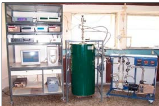
Fig. 23: fully automated low temperature (10-310 K) calorimeter
